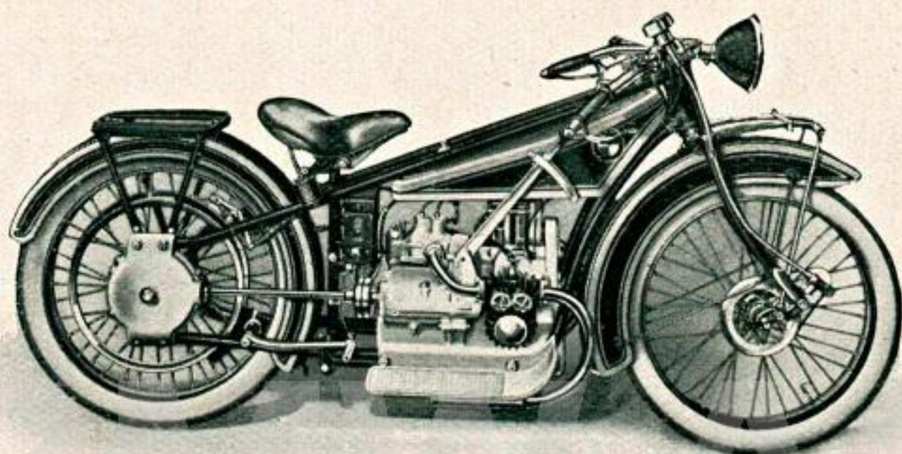
is produced by the Bayerische Motoren Werke in ever increasing series. Practically every one of its parts is made in the firm's own factories along lines which have caused world-wide repute to their products. The design of this road-worthy machine is a clear departure from the conventional rule of development from the old push-bike. It constitutes the successful solution of motor cycle construction on principles which, so far, have only been observed in motor car design.
