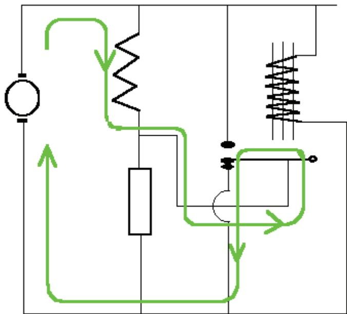
As long as the voltage is low enough, the regulator points are unaffected by the voltage coil. The current will flow from the rotor, through the field windings and the closed regulator points to ground. Thus the field windings get the maximum current.
