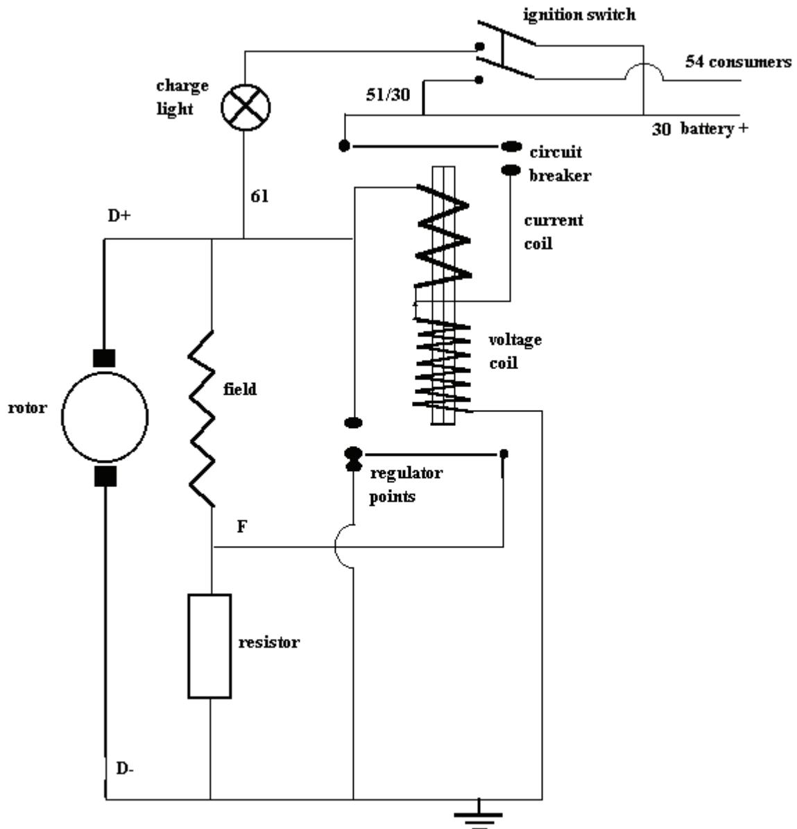
The complete diagram shows that there is also a current coil. This coil measures how much current is flowing from the dynamo to the battery and the other consumers. It acts on the same pair of points as the voltage coil. Its function is to drop the voltage as soon as the current rises too much.
