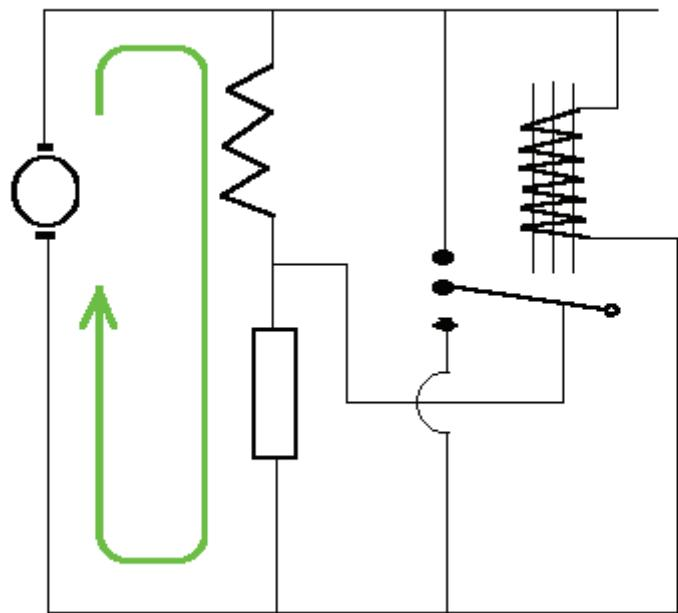
But as soon as the voltage rises above a certain level (7 - 7.5 Volt), the voltage coil pulls on the middle regulator point until it floats in the air. Now the current flows from the rotor, it can't go through the regulator points anymore, so it must flow through the resistor. The current is thus reduced, and the rotor voltage won't rise so fast anymore.
