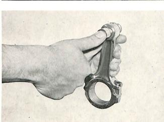
A correctly fitting wrist pin can be pushed through the bushing with light thumb pressure.
