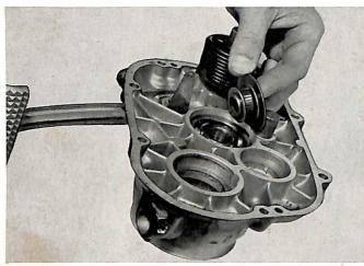
Remove bushing with shoulder from bearing. The determined cup shaped spacer (s) has to be placed on the bearing with the raised outer edge facing into the transmission. Reinstall bushing. The shoulder of the bushing must be included when measuring. We did so by installing it into the bearing before measuring.
