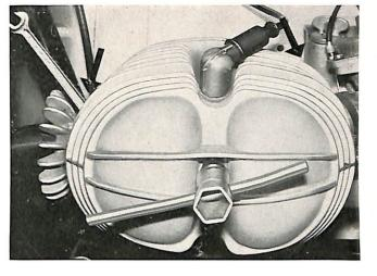
Remove the four (4) shoulder ruts and withdraw the rocker arms and push rods.
