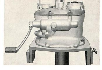
Remove speedometer cable hold down bolt and withdraw speedometer cable bushing with the help of two screw drivers. Remove speedometer drive gear.
