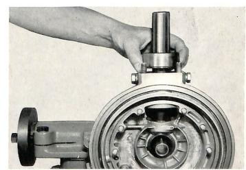
Tap off large ring gear ball bearing through the holes in the ring gear using a soft metal drift.
