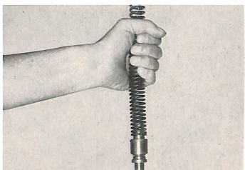
Loosen clamp nuts on lower fork yoke (for torque see ('Specifications'). Insert spreading wedge BMW tool No. 549 and withdraw fork tubes.
