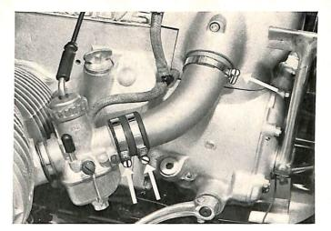
Remove the allenhead bolt in the center of the left air filter housing. Depress kick starter lever and remove filter housing.
