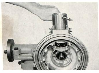
Remove threaded ring including seal with pin wrench, BMW tool No. 253. Remove inner spacer washer.
