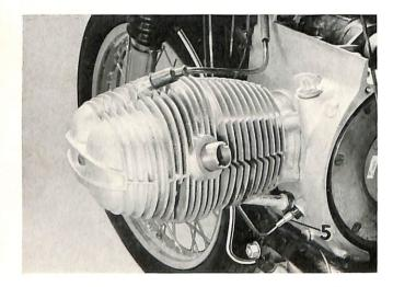
Withdraw front and rear engine through bolts
