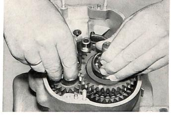
To measure the end play of the transmission shafts, install new gasket on transmission housing. Support output shaft with (fixture) BMW tool No. 504.
