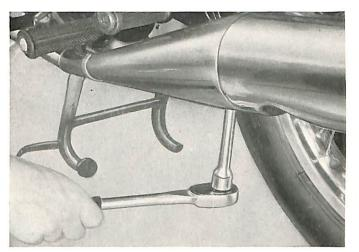
Loosen the allenhead bolts on the cross-over pipe and remove exhaust system.
