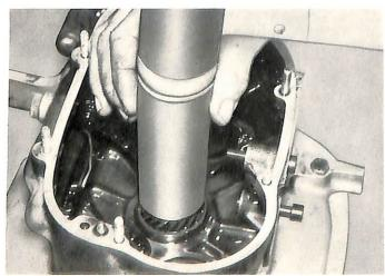
To install transmission shafts heat housing to 180—210° F. Place sleeve, BMW tool No. 206, on input shaft and insert input shaft into transmission housing. Under no circumstances should a hammer blow be directed against the end of the shaft. This would result in an improper fit.
