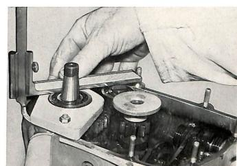
Measure the distance from housing cover mating surface to bottom of ball bearing seat in cover. Shim out the difference allowing for 0,1 mm (0.004") end play. The cluster gear is measured out exactly the same way, end play 0,1 mm (0.004"). During installation of the cover the shims can be held in the cover with a small amount of grease.
