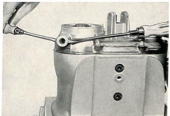
Bolt output flange holding fixture BMW tool No. 234 to output flange with four bolts M8 (hex.head size 13). Remove output flange nut (hex. head size 24 mm).
