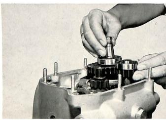
Mark the position of the eccentric bushing on each shift
