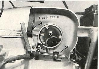
Remove the two allenhead bolts on the left and right and remove upper engine (starter) cover.
