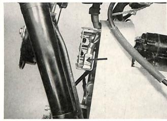
Remove left and right ignition wires an unplug wire from the oil pressure sensing switch (5)
