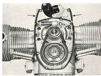
install guide bushing, BMW tool Nr. 225, into seal bore for advance unit shaft. Install timing case cover. Install allenhead bolts and nuts and tighten starting from the center to both sides.
