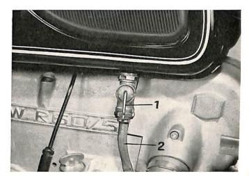
Flip up dual seat, remove wing nuts. Pull fuel tank to the rear then lift up at the front and remove.
