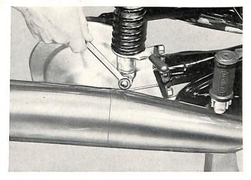
Drain oil from right swing arm tube. To facilitate draining remove filler plug also.
