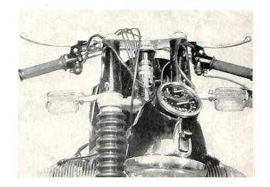
Remove allenhead clamp bolt from clamp ring (2). Loosen centering nut (1). Insert drift through the slot in the clampring into the split ring nut, tighten sufficiently to remove all play of the bearings. Tap lower fork yoke and center tube with a mellet to insure seating of the bearings. Tighten clamp ring (2). The steering head bearings are correctly adjusted if the fork falls to either side (with the clamp ring fully tight) of its own weight and no play can be felt in the bearings.
