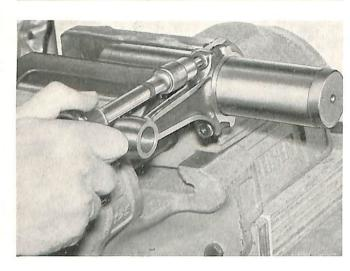
Measuring and straightening of connecting rods; Install a set of inserts into the big end (a set of inserts should be kept on hand to be used for this check whenever it is done) and mount the rod on a hardened ground mandrel. The rod should have no clearance on the mandrel. Insert a pin 150 mm (5.91") long, which fits without play, through the wrist pin eye.
