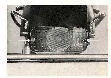
Remove the bulb from the reflector by pressing it in lightly and turning it to the left. It can then be withdrawn.
