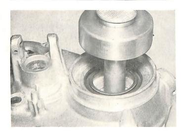
Remove clutch throw-out bearing and clutch push rod.
