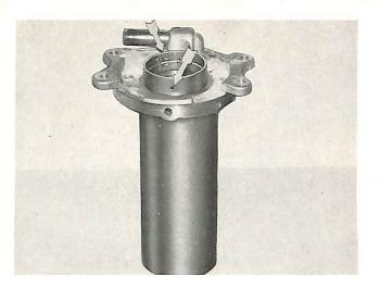
Clamp bearing retainer into vise (use jaw protectors). Drill two (0.126") holes into the bearing insert through the existing passages in the retainer. Carefully deburr holes in the insert.
