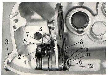
Slide segment (4) with selecting gear (5) on selector shaft (6). The selector lever engagement notches (7) have to have equal distance.from the selecting teeth on both sides. If necessary correct deviation by bending the return spring. Install pawl (8) on segment (4) install circlip (9). Secure segment with circlip (12) after installing detent spring (10) and washer (11).
