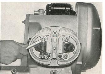
Install two shoulder nuts diagonally across on two cylinder through bolts. Install bracket BMW tool No. 209. Withdraw cylinder and cylinder head by tightening cap nut (hex. size 14 mm) on rocker box cover center bolt. As soon as the cylinder is free of the engine housing, remove the two nuts (hex. size 14 mm-see arrow) and separate cylinder from cylinder head with a light mallet blow. Withdraw cylinder head and cylinder from through bolts.
