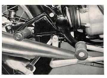
Rotate connecting pin to unhook the spring clip and withdraw it.
