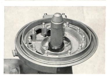
Pull needle bearing race from ring gear.
