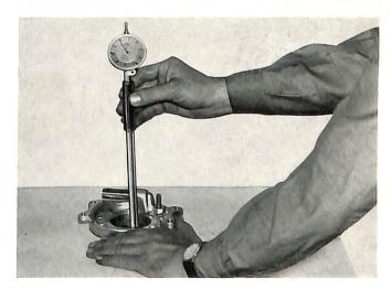
Bolt connecting rod caps and connecting rods together and measure in two positions using an inside micrometer. (For data see 'Specifications')
