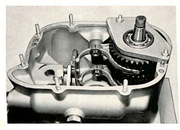
Check with inspection mirror and make certain that the the dewels are fully engaged into the sliding couplings, but that sliding couplings are not pressed against the
