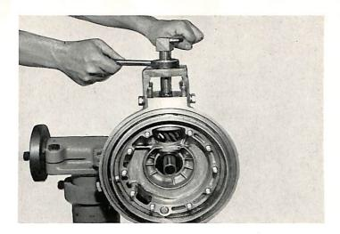
To replace pinion needle bearing, remove recessed pin, heat housing to 180° F. and remove bearing.
