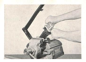
Pull drive shaft bell off. Use puller, BMW tool No. 204/2. Place a mandrel between puller spindle and drive shaft. If necessary direct a hammer blow against spindle to help remove coupling.
