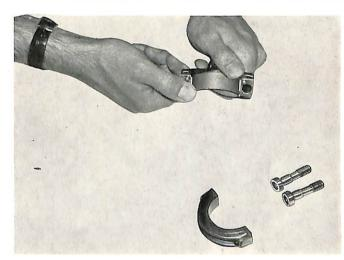
Before installation of the crankshaft, coat main and rod inserts with Molykote Paste "G".
