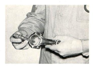
Check wrist pin bushing for tightness in the connecting rod, and check wrist pin for proper fit in the bushing. If the wrist pin has too much play in the bushing, replace the bushing.
