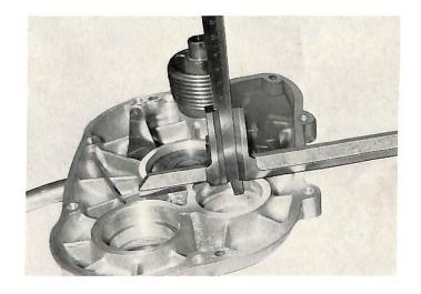
To facilitate measuring of the input shaft a 20 mm (0.8") bushing BMW tool No. 5061 is placed on the end of the shaft. Measure from the top of this bushing to the mating surface of the transmission housing. Subtract 20 mm (0.8") from the measurement. (This is the thickness of the bushing 5061).
