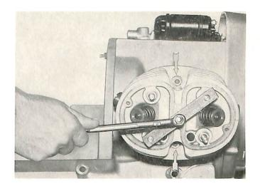
Assembly instructions; First place rocker arm alignment tool, BMW tool No. 200, on rocker arms. Tighten the six cylinder head nuts in the following sequence.
