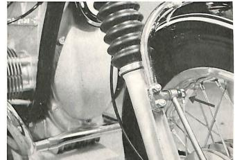
Remove axle nut (1) with washer loosen allenhead clamp bolt (2), and withdraw the axle (3).
