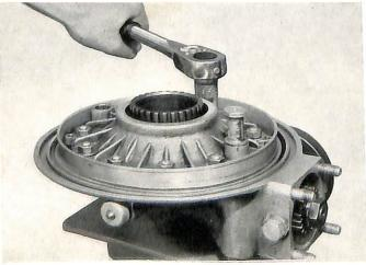
Using tool BMW No. 261, clamp rear drive unit into Workstand BMW No. 6000.
