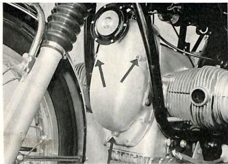
Loosen upper horn mounting bolt.
