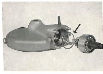
The difference between the two figures has to be inserted as shims between the rear drive housing and the pinion ball bearing (arrow).
