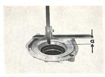
Adjust endplay to '0' without gasket. Use a depth gauge and a pair of prisms, BMW tool No. 50–36, and measure the distance from the ball bearing seat in the cover to the gasket mating surface of the cover (a).
