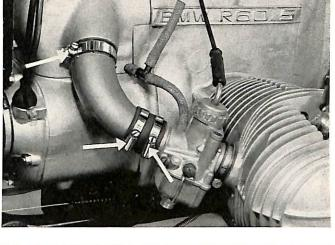
Loosen hex.nut (1) and hex.head bolt (2) of the right air filter housing. Remove filter housing, withdraw breather hose to the rear.
