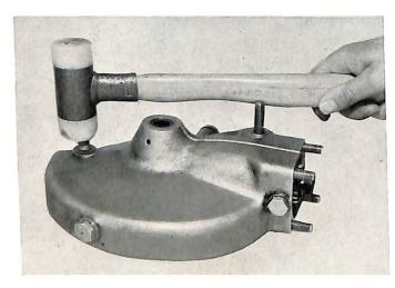
Remove nut from brake cam. Remove brake lever by tapping brake cam with a mallet inward.
