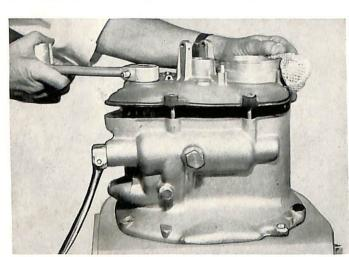
Heat transmission cover to 180—210° F. Place the shims for the shafts into the cover and install cover and output flange. For required torque see Specifications.
