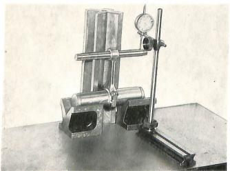
Lay two exactly alike prisms on a surface plate, place connecting rod vertical and measure the distance from the plate to the top of the pin at the wrist pin eye, to see if big end bore and wrist pin eye are parallel.
