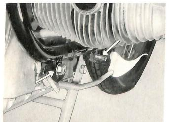
through bolt, place the center stand brackets between the engine housing and the frame on both sides. In addition the side stand bracket is placed between engine and frame on the left side.
