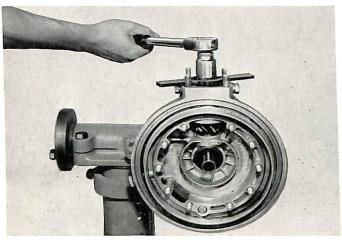
Remove lock tab, install holder BMW tool No. 256 and remove pinion nut. Withdraw drive pinion.
