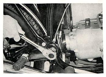
Remove swing arm bearing dust covers Loosen both lock nuts and remove both swing arm bearing pivot bolts. Observe torque requirements on reassembly (see 'Specifications').
