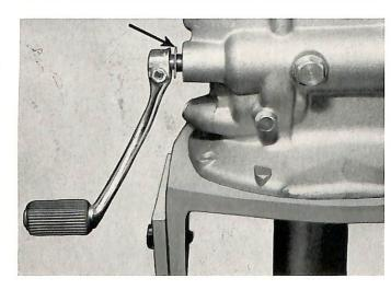
Install the foot shift lever, select the proper shims for the correct end play. Check Specifications.
