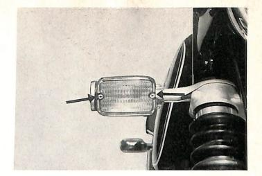
Disconnect the wire from the turn signal reflector (arrow).
