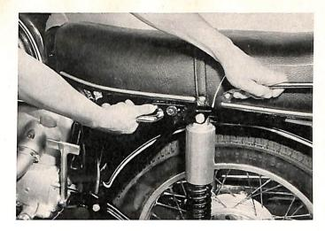
Remove the 3 allenhead bolts (arrow) and withdraw dual seat to the rear.
