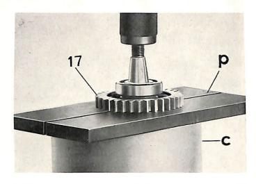
Place the divided plate p under the 1st speed gear (17), install the split plate upon an suitable press cylinder (c). Press off the speed gear together with thrust washer 19 and ball bearing 20.
