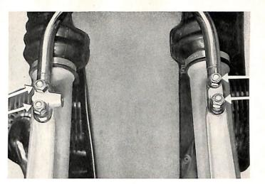
Remove the two nuts bolts and lock washers of the lower center brace.
