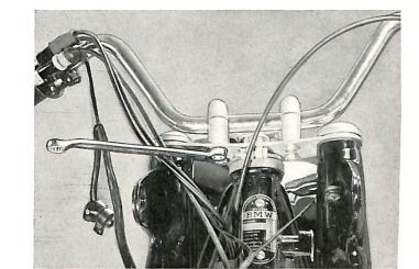
Remove upper aluminum fork covers with a pin wrench. Remove both upper spring retainers (for torque see'Specifications').
