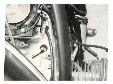
Remove hex.head bolt (arrow) with a socket wrench.
