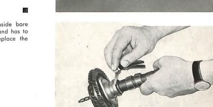
Checking end-play of camshaft. The assembly of the camshaft is in reverse order of the disassembly. Insert front camshaft bearing on camshaft, press on camshaft sprocket first and then press on tachometer drive gear, check end-play between camshaft bearing and camshaft with a feeler gauge. (For clearance see "Specifications".)
