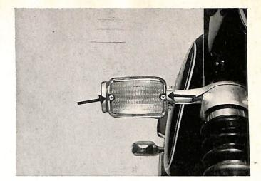
Remove bulb from reflector by pushing it in slightly and turning it to the left. It can then be withdrawn.
