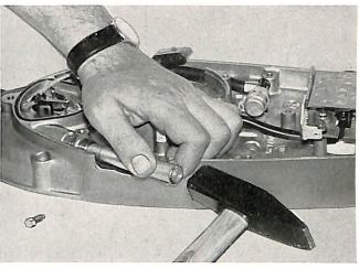
Installing timing case cover. Place crankcase in horizontal position. Lay gasket, and two sealwashers (arrow) on
