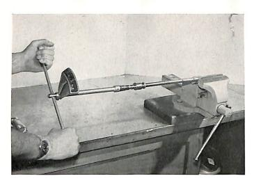
Assembly instructions: Reassemble shock absorber in reverse order. Clamp the hex, of the bottom retainer in vise and tighten both ends simultaneously by tightening at the hex. of the spring retainer. (for torque see 'Specifications').
