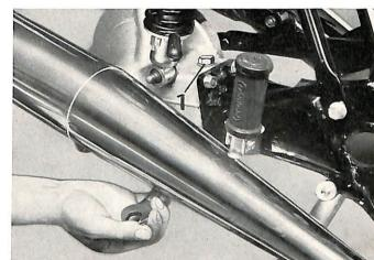
Remove wing nut from brake rod. Withdraw transverse pin from brake lever reinstall it on the brake rod and reinstall wing nut.
