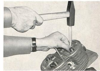
Install snap rings on new valve guides and press valve guides into heated cylinder head. (For fit see "Specifications"). Let cylinder heads cool down and ream valve guides with reamer 8H7.
