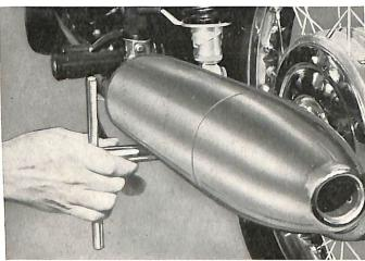
Remove clamp bolt on the left swing arm tube, and withdraw the axle.
