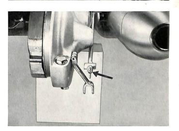
Loosen upper shock unit mounting bolt, remove the four nuts that hold rear drive to swing arm.
