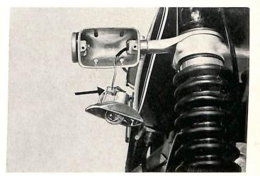
Loosen the clamp bolt and withdraw the turn signal housing.
