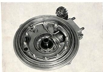
The base size of the gear set, measured from the pinion ball bearing to the center of the ring gear is  $75.5 \pm 0.05$  mm (2.97"  $\pm 0.002$ ").
