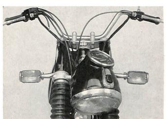
Remove handlebar brackets, protect fuel tank and lay handlebar carefully on tank.
