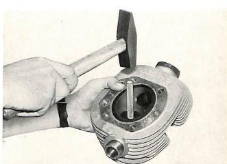
**Refacing valve seats:** Reface the valve seats in the cylinder head with the "Hunger" or another suitable seat refacer. The valve seat face has an angle of 45° 20'. The seat width is 1,5 mm (0.060") for the intake valve and 2,0 mm (0.080") for the exhaust valve, measured at a 45° angle. Chamfering toward the combustion chamber should be 15°, chamfering toward intake or exhaust port should be 75°. The seat at the valve should be positioned near the outer diameter.
