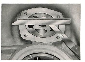
Check clearance between inner and outer rotor. (for clearances see "Specifications")
