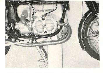
Remove the cotter pin and remove the nut from the allenhead bolt which holds the brake support arm. Withdraw the bolt.
