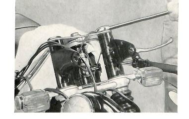
Remove centering nut and remove upper fork yoke. (for torque see 'Specifications').
