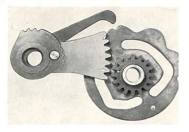
The over-shift ([a] between pawl and detent notches) is determined by the selector gear limiting bolts. The overshift should be 1 mm (0.04") in 4th gear on the upshift and on 1st gear on the downshift. If necessary correct this by shimming.limiting bolts.
