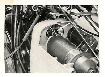
Unplug the wire on the left side of the diode chassis
