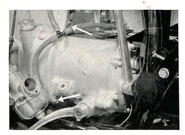
Unhook clutch cable on transmission. Remove the through mounting bolt bottom right, the longer bolt on top and the shorter bottom bolt.
