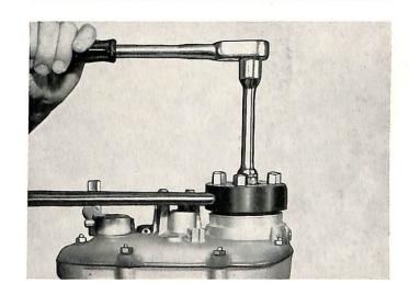
Install output flange puller BMW tool No. 232 with four bolts M8 $\times$ 1 (hex.head size 13 mm) and pull off output flange I necessary place a light hammer blow onto the puller spindle.
