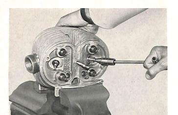
If necessary lap in valves using holder, BMW tool No. 540.
