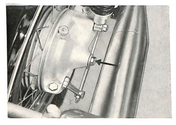
Remove axle nut and washer.
