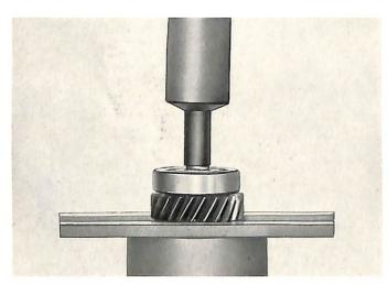
Remove circlip (2) from the forward end of the output shaft. Place two bars between fourth gear (6) and sliding coupling (8). Press off bearing (3) with appropriate mandrel.
