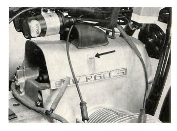
Unhook the battery straps, remove battery cover and disconnect negative battery cable.
