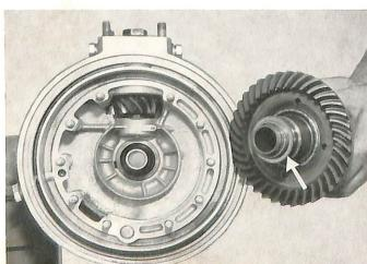
To adjust the backlash, place an appropriate size brass thrust washer between the needle bearing inner race and the needle bearing of the ring gear.
