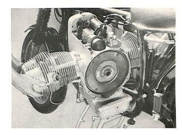
Install the engine on work stand BMW No. 6000 in device BMW No. 6005/1 and fasten by screws. Prior to disassembling the engine, it's good practice to check ignition timing 12 11 004, contact breaker points gap 12 11 141 as well as the value clearances 11 34 504 in order to localize previously existing faults and to hold them in mind on further checks.
