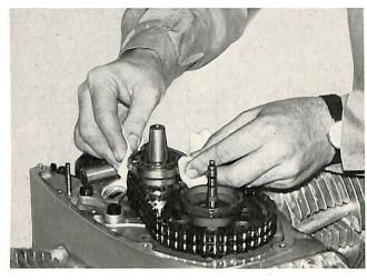
Tighten front camshaft bearing with two phillips head
