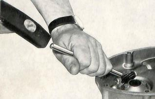
11 14 800 Timing case cover removal and installation
