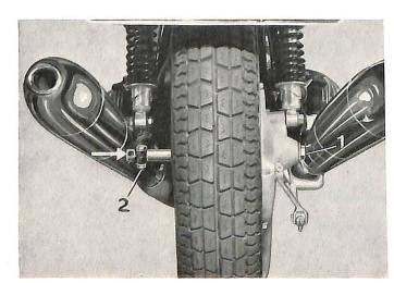
Assembly instructions: Clean the axle and splines; grease lightly with a high drip point grease. Rotate axle during insertion. After tightening the axle nut (1), take the motor cycle from the center stand and depress the rear end several times to prevent binding, then tighten clamp bolt (2)—the hole in the end of the axle (arrow) should be horizontal.
