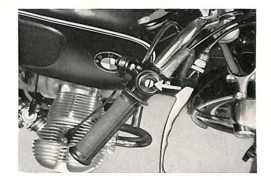
Assembly instruction: Before assembling grease throttle cam and grip. Line up end of slot 'b' with end of opening 'a'. Insert bottom throttle cable into cam chain and insert cam into throttle assembly so that markings 'c' and 'd' line up. Insert upper throttle cable and pull outer cable back far enough to be able to install cover. Tighten cover and push up rubber cover.
