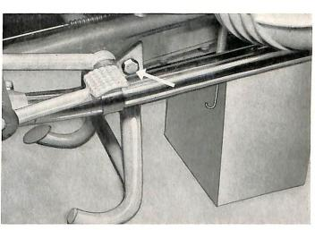
Remove hex head bolt (left and right) (arrow) and withdraw center stand to the rear. Watch for the spacers.
