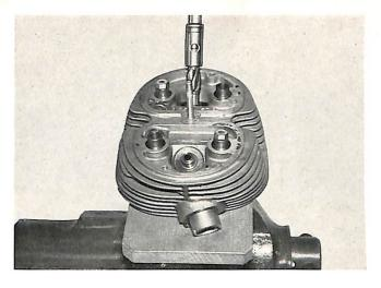
Remove snap ring, heat cylinder head to 360° F and drive valve guides toward combustion damper using drift, BMW tool No. 5128.
