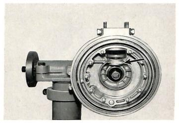
**Assembly instruction:** Install pinon needle bearing with drift, BMW tool No. 252.
