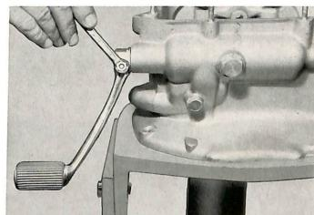
4) Remove shift selector assembly with bushing, holders, circular leaf spring, washer and return spring. Reassemble in the following order. 1. Install bushing on shift selector assembly with the
