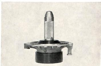
Heat housing to 180° F and remove needle bearing.
