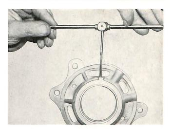
Clamp installation mandrel with fiber sleeve into vise. Put cover over mandrel and tap in locating pin far enough that it recedes  $0.02 \div 0.04$ " from the inner bearing surface. Centerpunch pin in place and carefully deburr hole.
