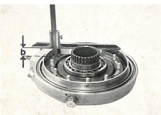
With the ring gear installed in the rear drive housing, measure the distance from the ball bearing to the gasket mating surface of the housing (b). (This is done without the gasket).
