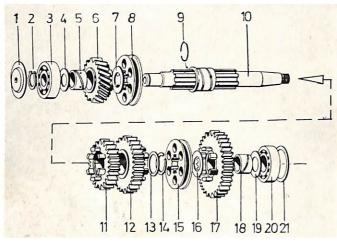
Remove floating bushing (18) of first gear, second washer (16) sliding coupling (15) for first and second gear.
