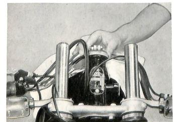
Remove headlight brackets with the rubber rings and withdraw the turn signal wires. (the lower fork yoke has vent passages and holes for the turn signal wires).
