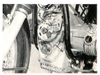
Loosen upper horn mounting bolt. Unscrew the three allen head bolts and remove front engine cover
