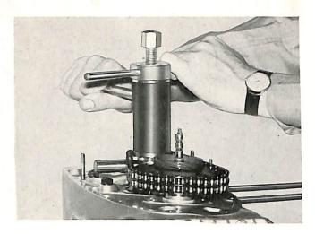
Insert camshaft into engine housing - push crankshaft sprocket on crankshaft carefully so that key and key groove mate. Install fixture sleeve, BMW tool No. 216, and puller bolt, BMW tool No. 535, over sprocket into the end of the cranshaft and pull the sprocket on.
