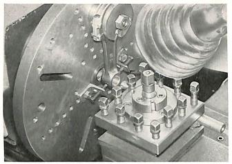
Press new wrist pin bushing in. Mount connecting rod in a lathe and turn bushing to a high finish to the proper size. (See Specifications)
