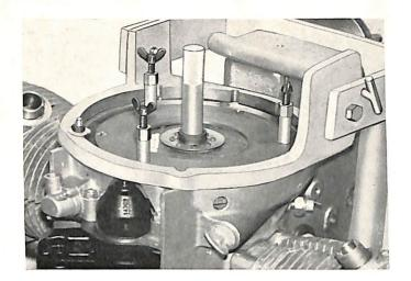
During reassembly use centering arbor, BMW tool No. 529, to properly position the clutch plate.
