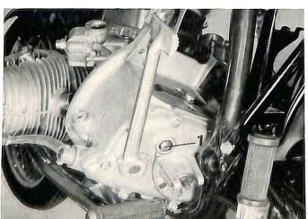
Remove transmission partially to the left and disconnect the neutral indicator wire.
