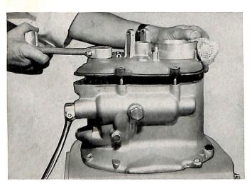
To install cover, heat it to 180 to 210° F. Place it on the transmission and depress kick starter partially. Move the kick starter up and down slightly to engage kick starter gear.
