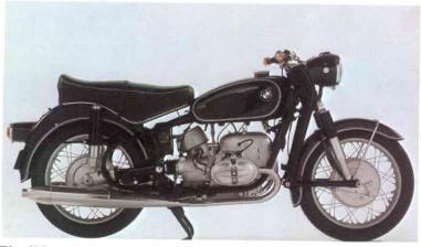
The "German School" of motorbike construction is now more than 40 years old. But every BMW still incorporates the decisive features of the revolutionary principle of 1923 — the closed double-tube frame, the transverse horizontally-opposed motor, the unitized motor-transmission construction, and the elegant shaft drive.
