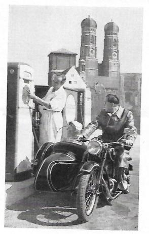
out hub spindles. Other advantages worth mentioning are the following: The sidecar is easy to enter and offers ample leg room; comfortably upholstered seat with high back; dust-tight apron with removable "Cellon" plastic windscreen gives full protection; luggage easily accommodated in and on rear section.
