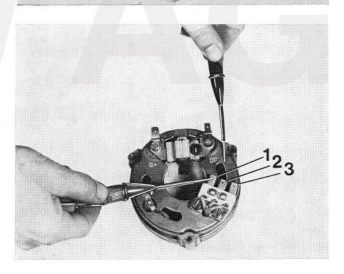
Check the resistance alternatively between the phase outputs, see Technical Data section for values.
