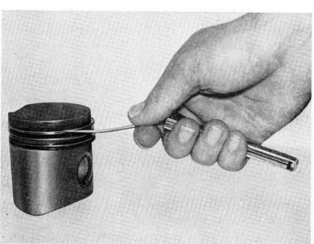
and side clearances of the piston rings with the aid of a feeler gauge. See the Technical Data for the nominal dimensions and oversizes of cylinder bore and piston, diameter and the ring gap and side clearances of the piston rings.
