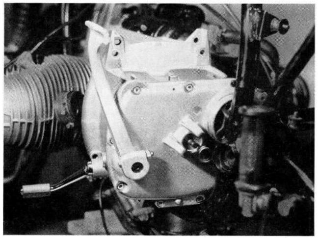
Take off the from the swinging arm mounting. Slacken the locknuts to the left and right of bearing journals and unscrew both bearing journals.
