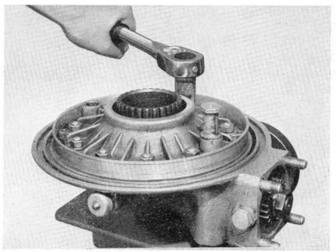
Draw the rear wheel drive off the swinging arm and lay aside.
