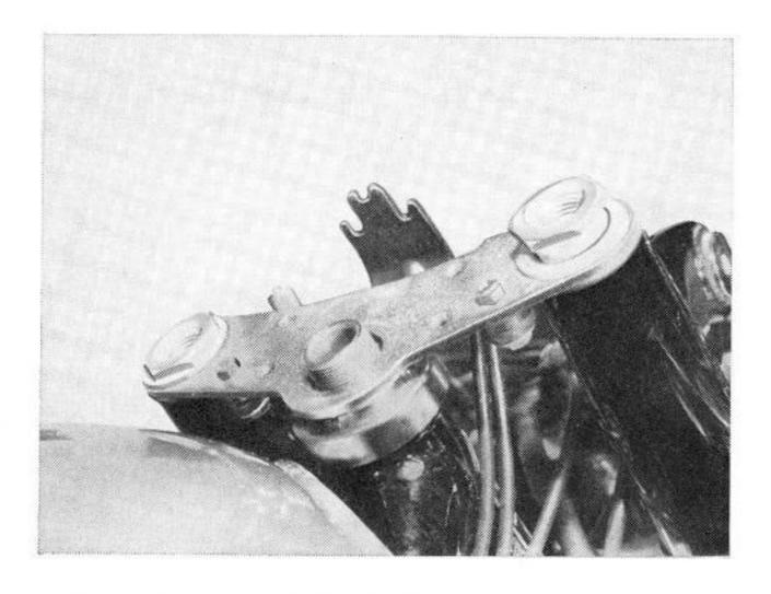
Unscrew the two upper spring seatings with their shims (see Technical Data section for tightening torque) and take off the upper fork yoke.
