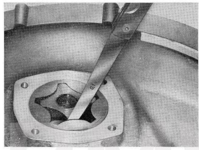
Determine the gap between the inner and outer rotors with the aid of a feeler gauge. See Technical Data section for clearances.
