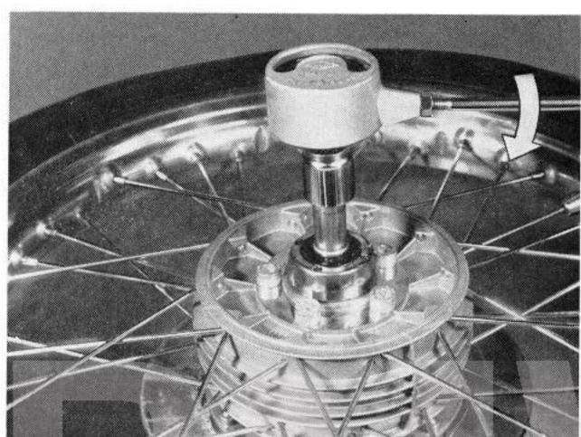
Press the guide sleeve out of the cap. Push the bearing off the sleeve.
