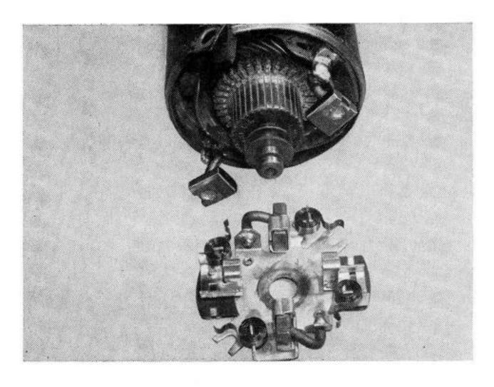
Lift out the positive brush and remove the brush holder plate.
