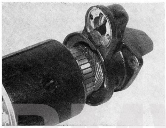
Separate the pole housing from the drive bearing.
