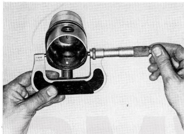
Use a micrometer gauge to measure the piston diameter at the piston skirt transverse to the wrist pin bore.
