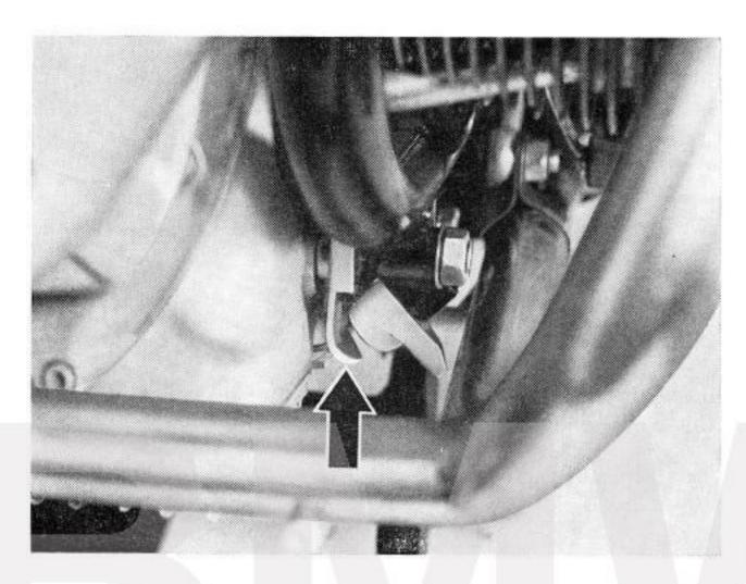
Remove left-hand hexagon nut of front engine mounting. Knock through the engine bolt so that the shackle (arrow) can be taken out.
