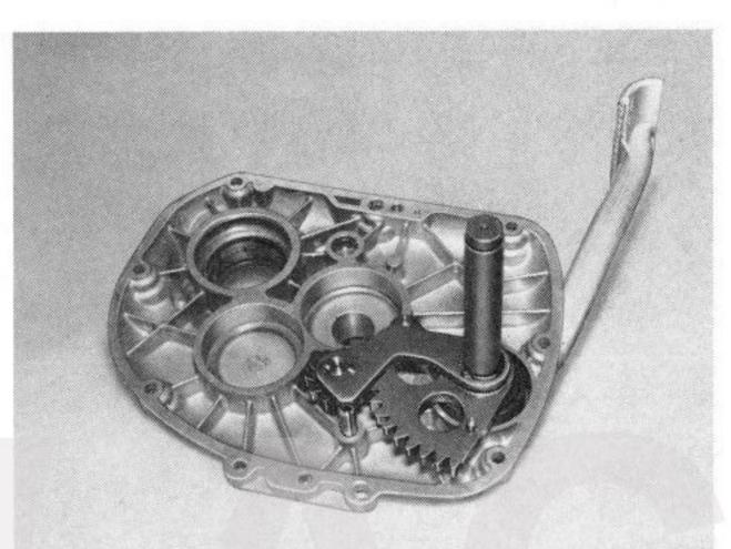
Remove the circlip for the intermediate gear and take off the intermediate gear of the kick starter.
