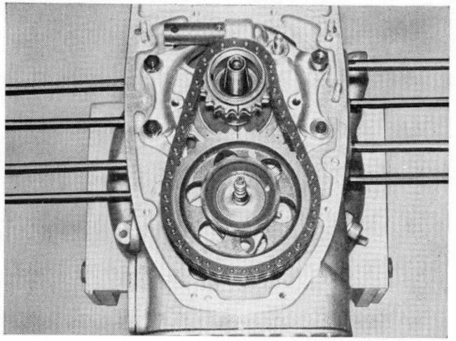
Insert the camshaft into a suitable pipe (outer diameter approx. 106 mm, inner diameter approx. 90 mm and length approx. 225 mm) so that the sprocket lies flat on the pipe. Fit BMW No. 212 sleeve on the camshaft end face and press out the sprocket together with the rev. counter drive gear.
