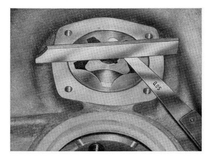
See Technical Data section for clearance between pump housing contact surface and rotor sealing surface.
