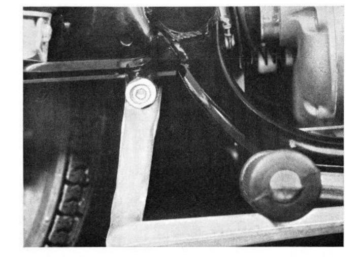
Detach the ES bolt from the brake pull rod and remove pull rod.
