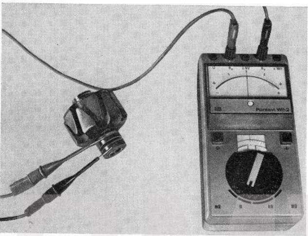
Check energizer winding (ohmmeter).
