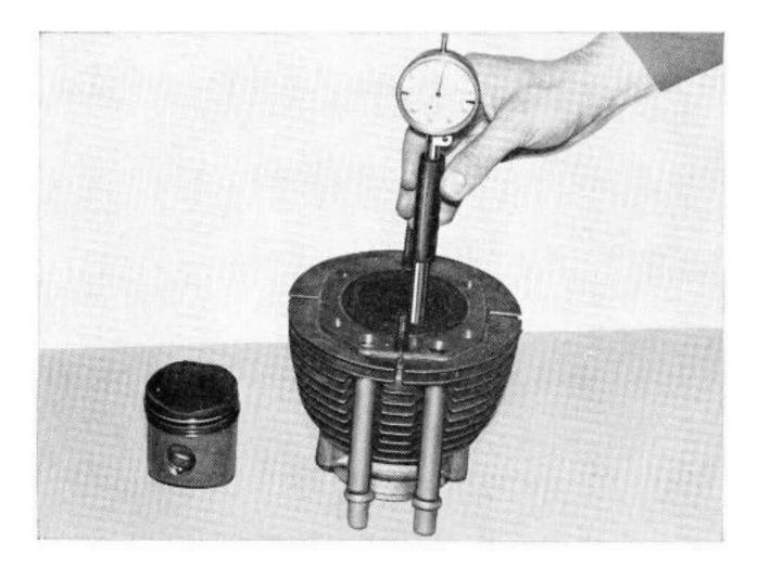
**Testing and Repair:** Measure the cylinder bore in the wrist pin direction and at 90° thereto 10 mm from the top, in the centre and at the bottom with an inside gauge. This should be carried out at a room temperature of 20° C.
