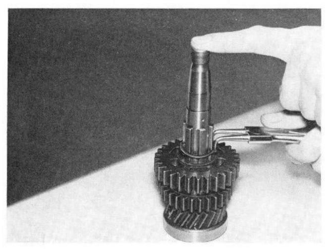
Unscrew Phillip's screw for oil guide cover and remove cover. Withdraw shaft for selector forks 1-2-5 and remove forks.
