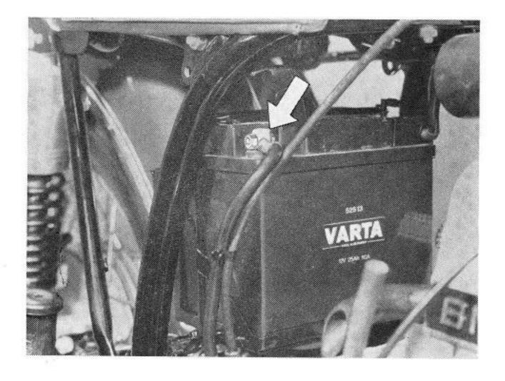
Disengage the battery clamping straps, lift cover upwards and
