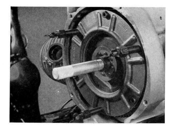
When re-assembling use the BMW 529/1 centring arbor to locate the clutch plate. See Technical Data section for tightening torques.
