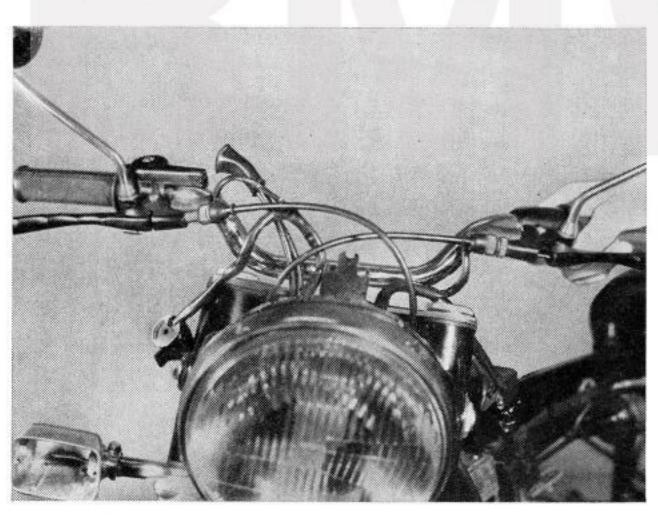
Note when fitting: When refitting care must be taken to ensure accurate positioning of the control cables.
