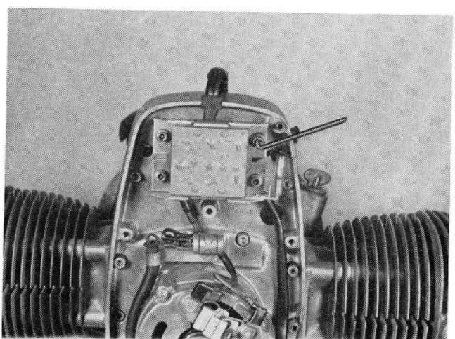
Check the diode carrier after removing the flat plug.
