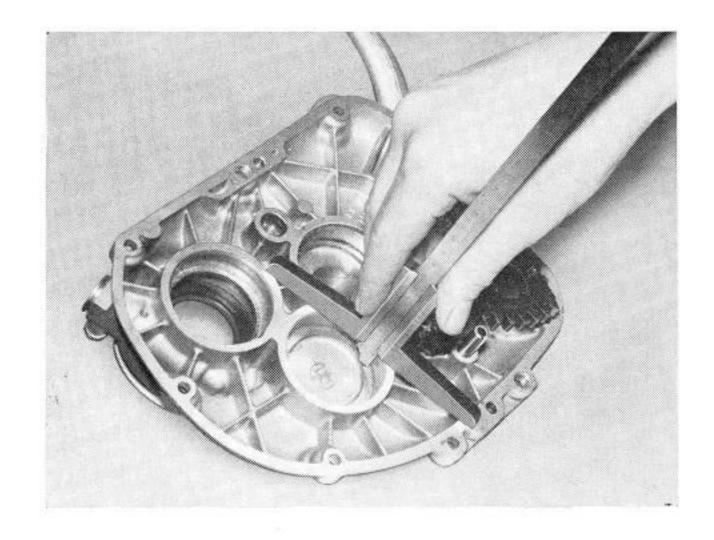
Now measure the distance between the housing cover contact surface and the base of the ball-bearing seating in the cover and compensate any discrepancy with appropriate shims down to a clearance of 0.1 mm. It is advisable to stick the shims in the bearing seat of the gearbox with the aid of a little grease.
