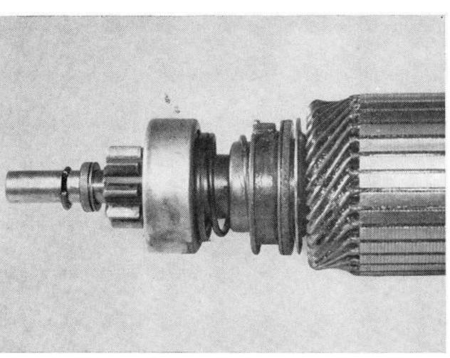
Press the thrust ring to the rear. Lift out circlip. Pull off starter gear.
