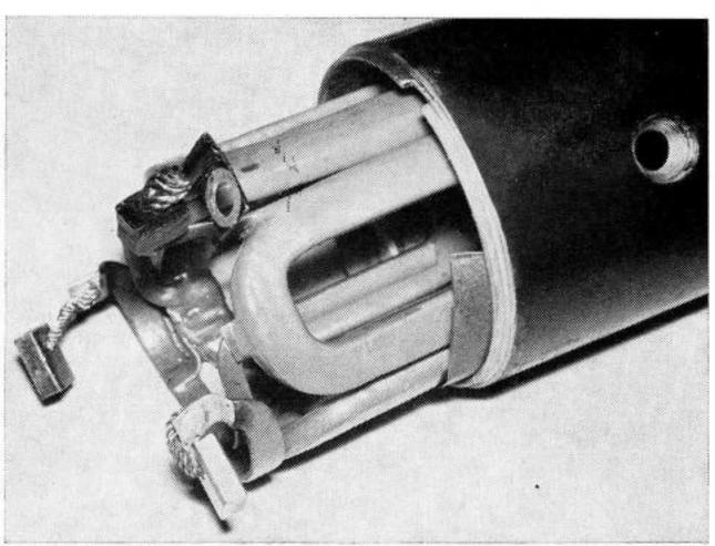
Superfinish the commutator. The commutator diameter (A) may not be less than 33 mm.
