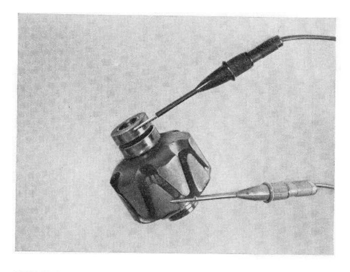
After removal, check the claw pole rotor with 40 V ac for shorting.
