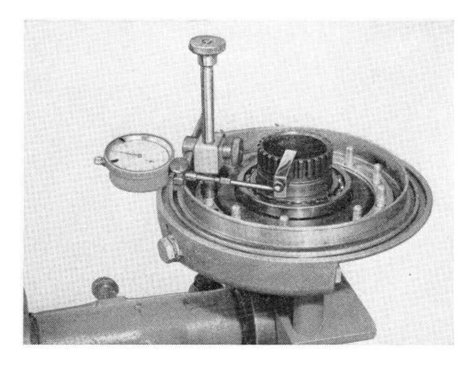
Check the gear mesh and backlash (see Technical Data section) around the outer diameter of the crown wheel with a dial gauge and BMW jig No. 5104 with BMW clamp No. 260.
