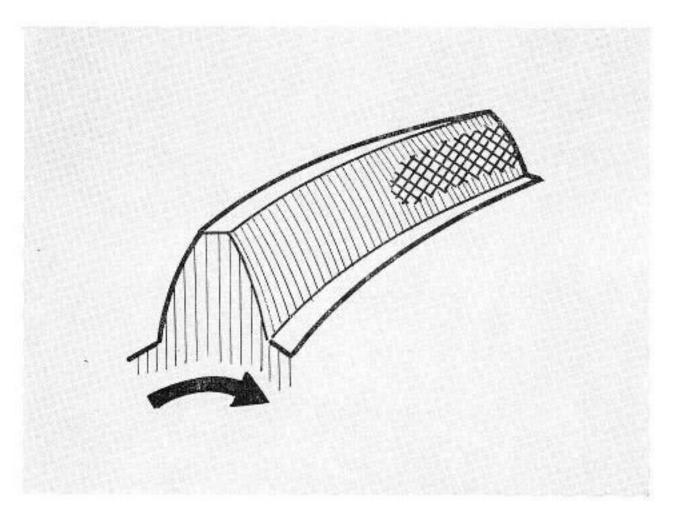
If the contact pattern lies at the thinner end of the tooth the pinion spacing from the crown wheel centre will have to be reduced by the use of thinner shims at the ballbearing outer race and the tooth backlash corrected by a thicker bronze shim at the needle bearing.
