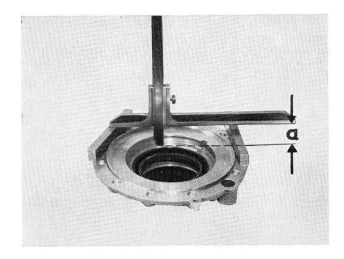
On the rear wheel drive housing, without a gasket on the contact surface, measure the distance (b) of the grooved ball-bearing on the crown wheel to the contact surface. Play can be eliminated by fitting an appropriate number of shims between the grooved ball-bearing and the seating base in the cover. The required shim thickness is obtained by deducting dimension (b) from dimension (a). The required play is obtained after fitting the gasket; the crown wheel must not be under pressure.
