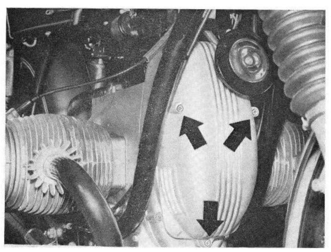
Slacken the top fastening screw on the horn.
