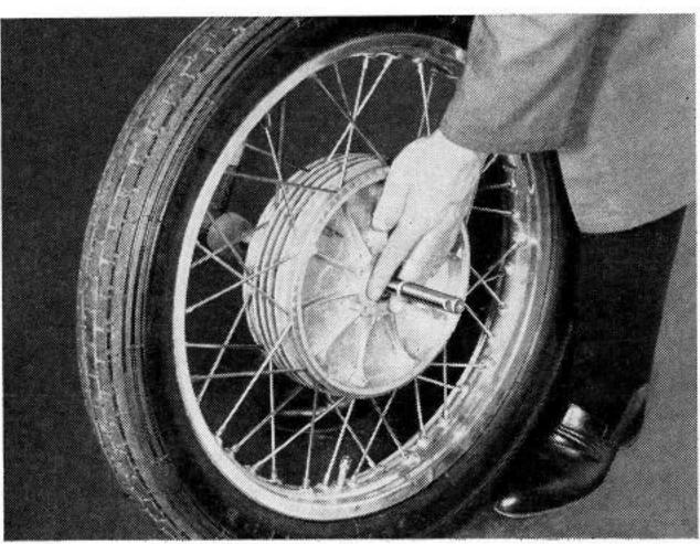
Maximum radial and lateral run-out measured at rim flange (see Technical Data).
