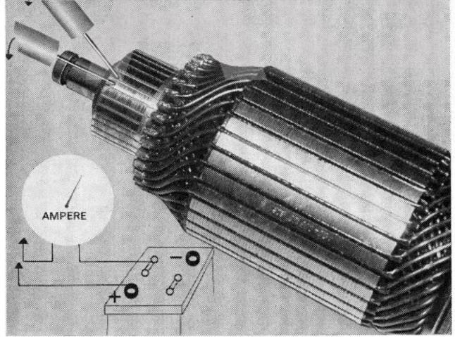
Check energizer coil for earthing. Replace scorched or charred windings.
