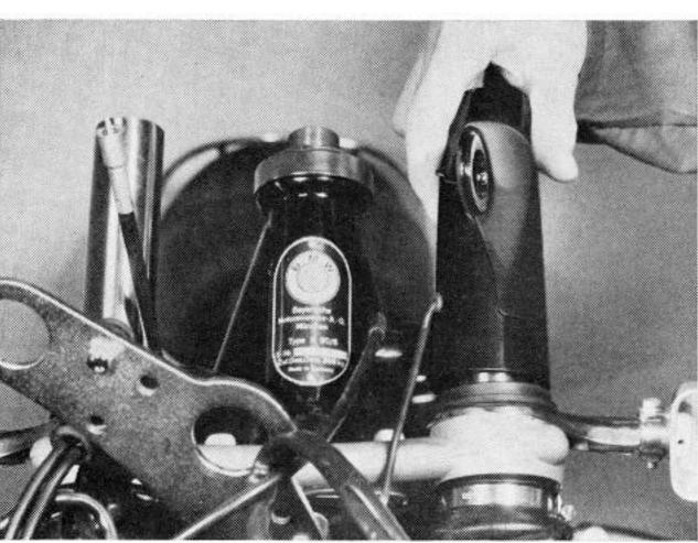
Remove headlamp mounts left and right with rubber rings and turn indicator leads (the bottom rubber rings are provided with bores for breather capillaries in the fork yoke and bores for leads to the turn indicators).
