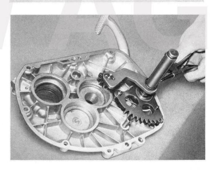
Loosen the splined bolt of the kick starter lever and remove lever. Lift out the kick starter from the cover with the washer and spring.
