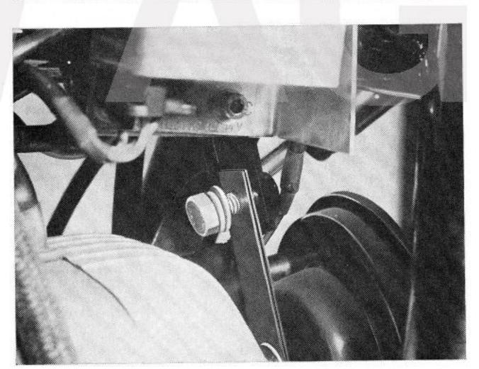
Pull off protective rubber sleeve. Disconnect leads from horn.
