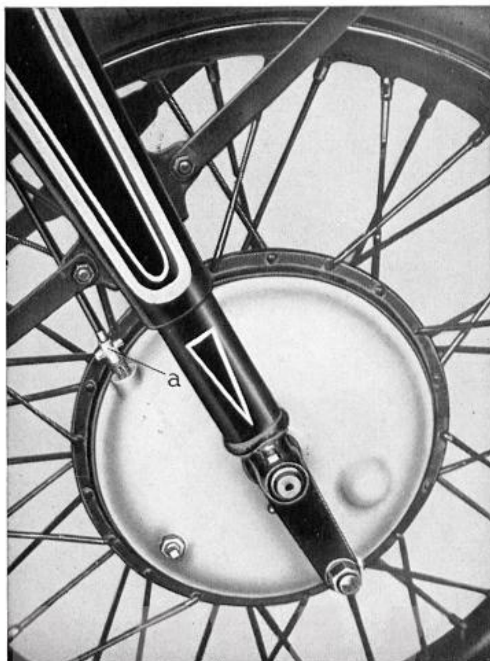
Fig. 7 Front wheel brake
